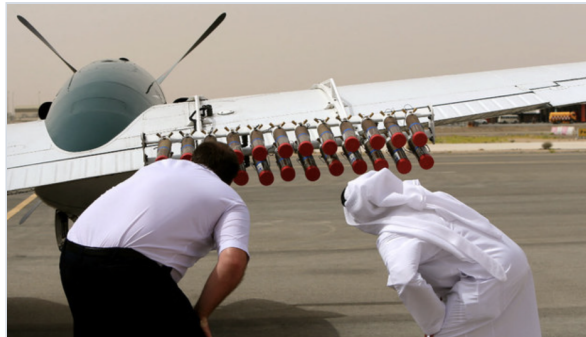
UAE rain-enhancement drone with electric-charge emitters. Image: from the 8th book
