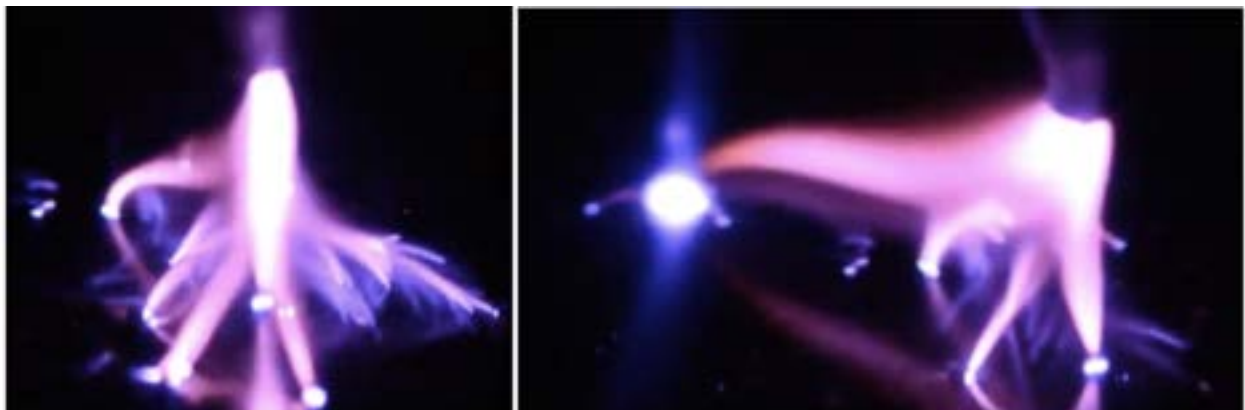
ABOVE: (Left) Current into granite. (Right) Cracks in granite become illuminated with plasma. BELOW: More examples, with the lights off.
